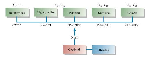
**FIGURE 2.2** Distillation of crude oil yields a series of volatile fractions having the names indicated, along wih a nonvolatile residue. The number of carbon atoms that characterize the hydrocarbons in each fraction is approximate.
