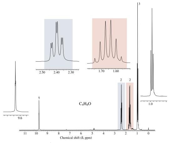
FIGURE 17.17 The 200-MHz <sup>1</sup>H NMR spectrum of a compound (C<sub>4</sub>H<sub>8</sub>O) (Problem 17.43).
