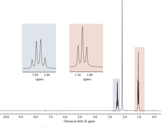
FIGURE 17.15 The 200-MHz <sup>1</sup>H NMR spectrum of 2-butanone. The triplet-quartet pattern of the ethyl group is more clearly seen in the scale-expanded insets.
