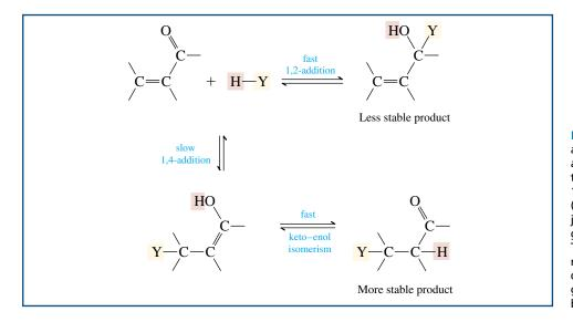
**FIGURE 18.6** Nucleophilic addition to  $\alpha$ , $\beta$ -unsaturated aldehydes and ketones may take place either in a 1,2- or 1,4 manner. Direct addition (1,2) occurs faster than conjugate addition (1,4) but gives a less stable product. The product of 1,4 addition retains the carbon–oxygen double bond, which is, in general, stronger than a carbon–carbon double bond.
